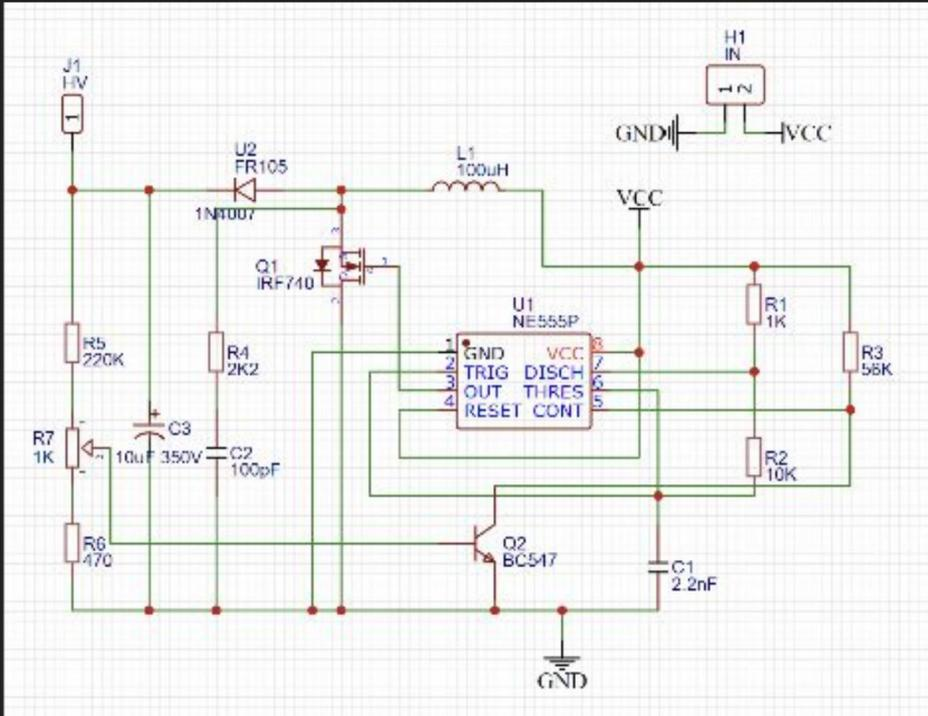
The very popular **555 timer**, whose period and duty cycle is controlled by the capacitor **C1** and the resistors **R1**, **R2**, generates a square wave given to **MOSFET Q1**.
