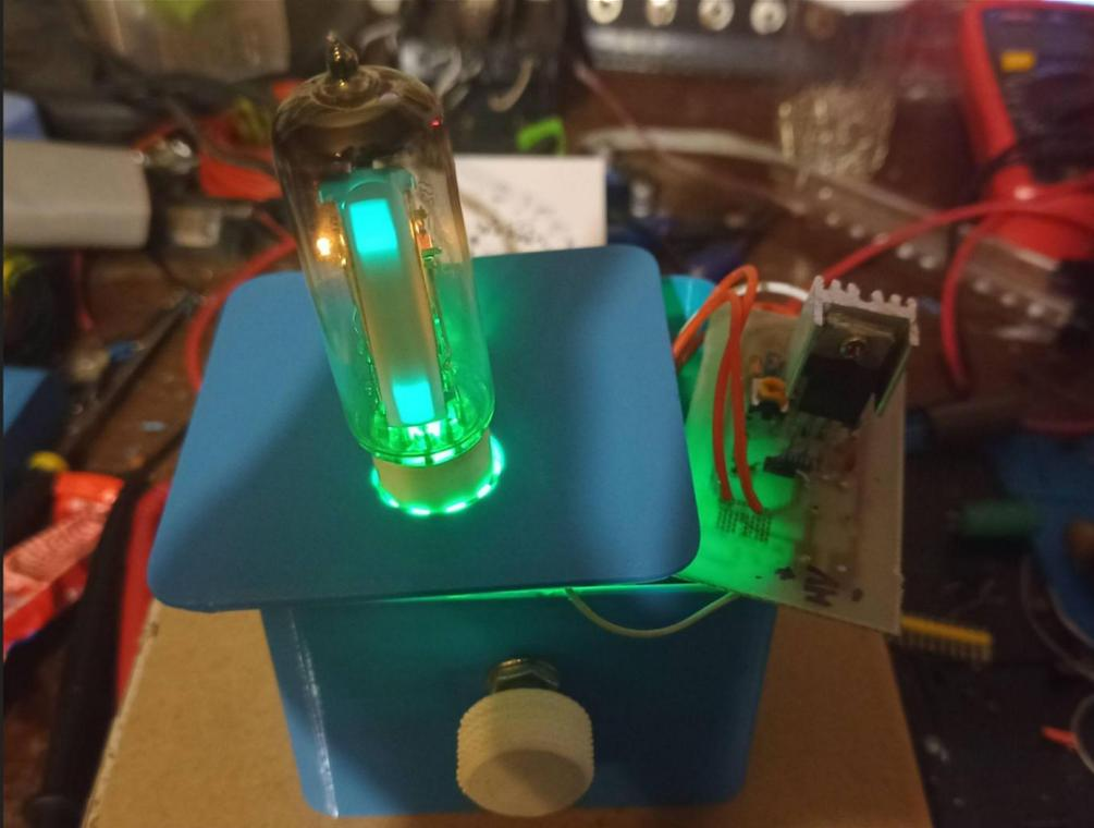
I used this converter to power the "maic eye" **6E2 vacuum tube** (EM84 replacement).
