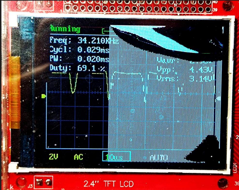
Ignoring the damage to the "toy" screen of the oscilloscope, you can clearly see the waveform that the 555 generates.
