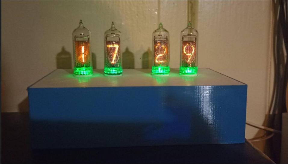
I made a practically identical circuit and used it to power the **Nixie 1N-14** tubes (**IN-14** after "ours") in the clock.
